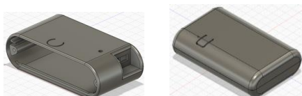
Fig. 4 Solid models of sensor case by 3D-CAD
