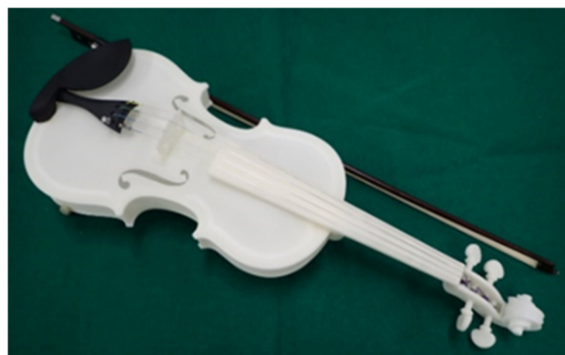
Fig.4 The additive manufactured violin
