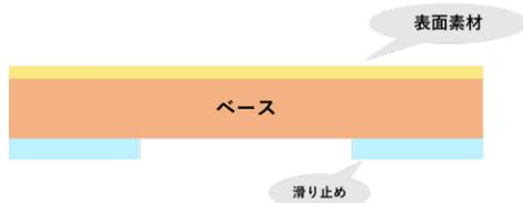
Fig.10 Structure of the Prepared Evaluation Samples
