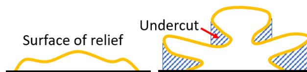
Fig. 2 Cross sections of bas-relief (left) and high-relief (right).
