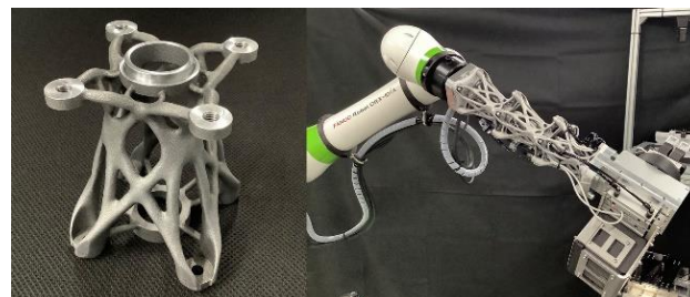
Fig. 3 "Arm Block" manufactured by AM
