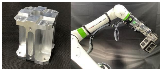
Fig. 1 "Arm Block" manufactured by cutting
