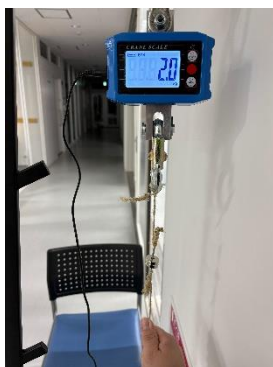
Fig 5. Test setup for pull-off load with a screw-fastened magnet.
