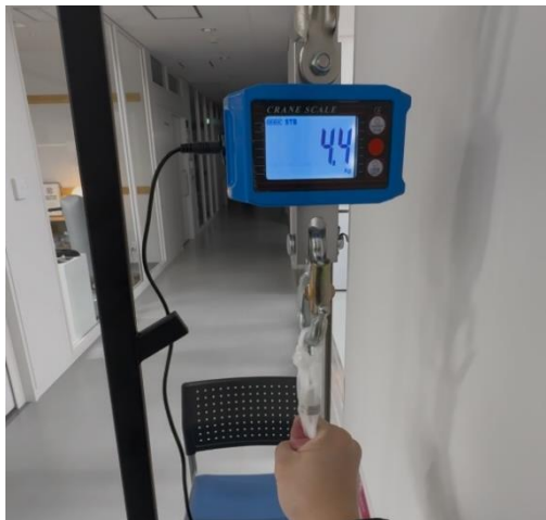
Fig.1 Setup for measuring the pull-off load of magnets
